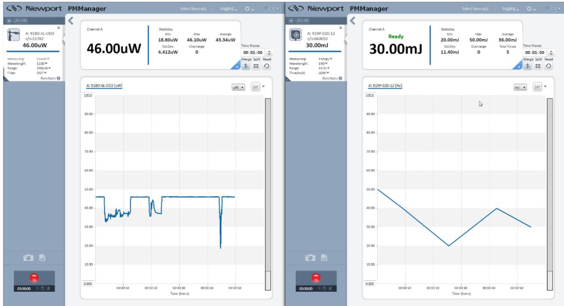
This display method may have a purpose when certain time-related analyses are required because each X-axis can have its own definition. Each channel is given the same default color. However, the method does not allow performing Math Channel operations between two channels. Only operations on the same channel are available. See [Math Channels](#). Moreover, the option to Capture Screen, outputs only the selected channel and not both channels.
